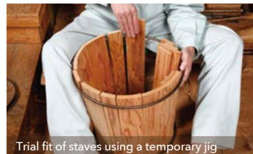
Trial fit of staves using a temporary jig
