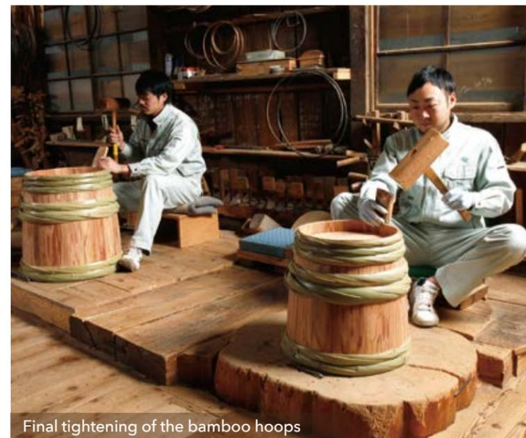
Final tightening of the bamboo hoops
